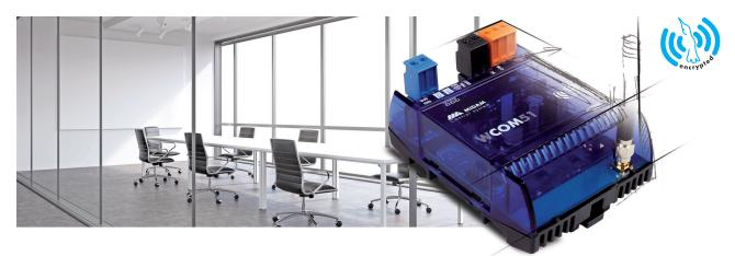
Router/repeater for integration of up to 50 wireless devices. The communication is based on the AES 128 encrypted Midam KFP protocol, which allows to update the device firmware on a wireless basis across the wireless network topology. Native modbus map grants seamless integration into the DDC/SCADA systems. Thanks to the "dual stack radio" technology, it can read values from wMbus based devices simultaneously.
